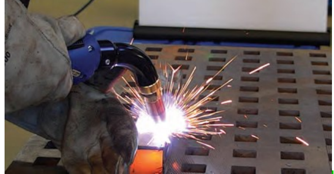
Fume Extraction Source Capture Suction is ON
